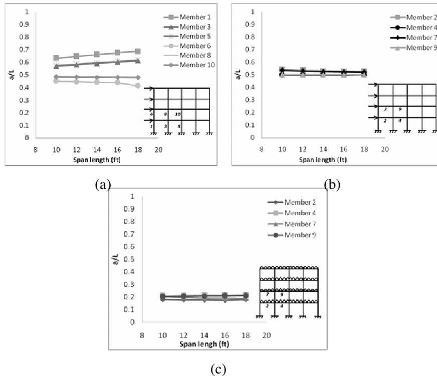
Figure 16: Variation of  $a/L$  with Span length (a) and (b) for lateral load (c) for UDL.
