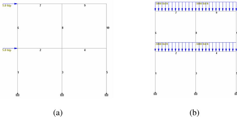
Figure 6: Plane Frames (a) with lateral load (b) with uniformly distribute load (UDL).
