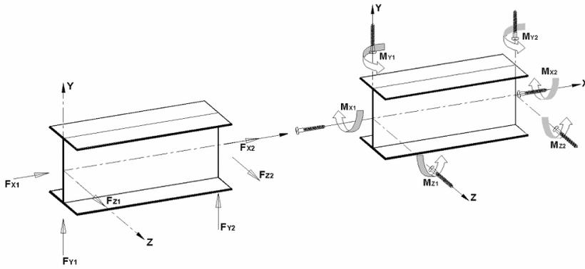
Figure 5: Member end forces and moments in STAAD.Pro 2006 environment (Bentley Systems Incorporated, 2006)
