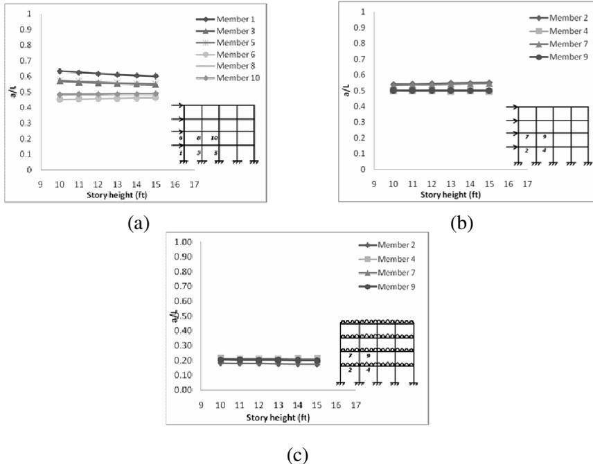
Figure 17: Variation of  $a/L$  with Storey height (a) and (b) for lateral load (c) for UDL.
