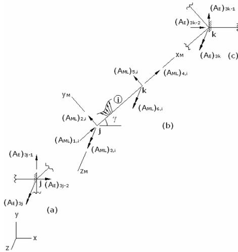
Figure 4: Loads on plane frame member
