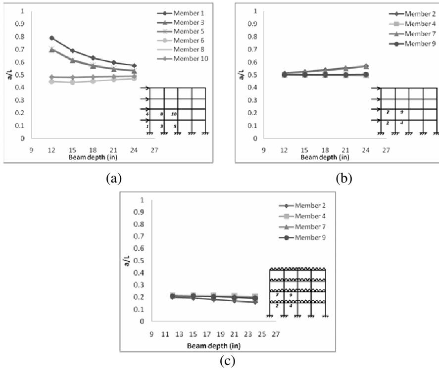
Figure 15: Variation of  $a/L$  with Beam depth (a) and (b) for lateral load (c) for UDL
