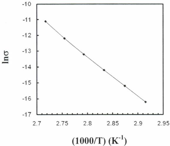
Fig.6 Variation of  $\ln\sigma$  versus  $(1000/T)$  for CdSe thin films prepared at  $200^{\circ}\text{C}$ .
