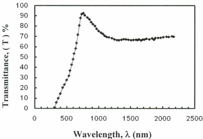
Fig 1. Optical transmittance T(%) at different photon wavelength of CdSe thin films prepared at  $200^{\circ}\text{C}$ .
