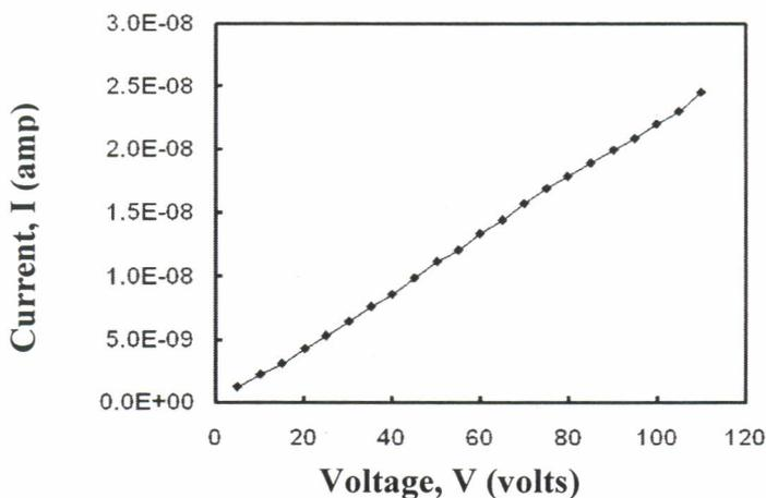
Fig.4. I-V characteristics of CdSe thin films.
