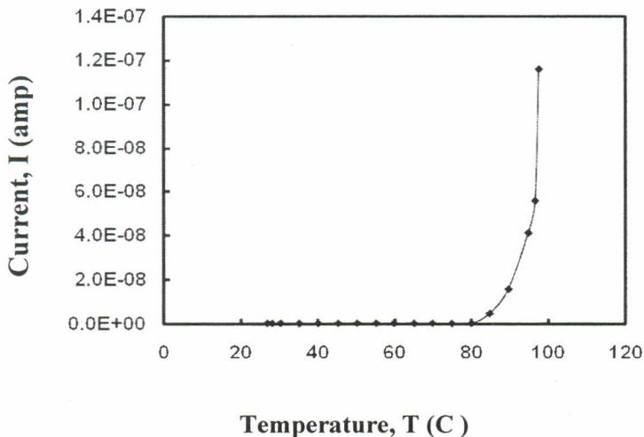
Fig.5. The dependence of current I (amp) on temperature T(C), of CdSe thin films prepared at 200° C.
