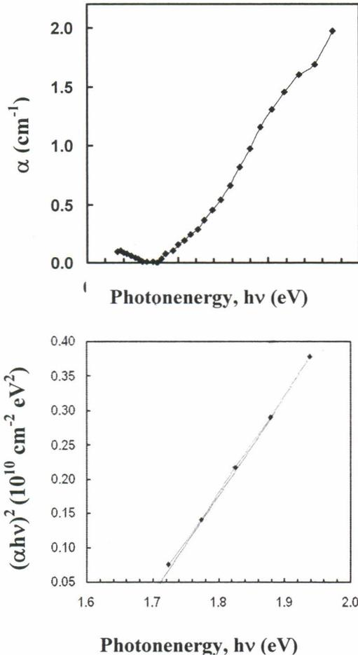
Fig. 3 The dependence of (a) absorption coefficient,  $\alpha$  and (b)  $(\alpha h\nu)^2$  on photon energy ( $h\nu$ ) of CdSe thin films, deposited simultaneously from elemental (Cd and Se) sources at  $50^\circ\text{C}$ .
