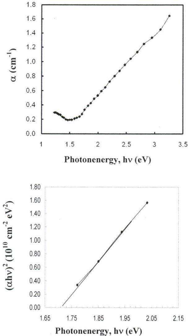
Fig.2 The dependence of (a) absorption coefficient,  $\alpha$  and (b)  $(\alpha h\nu)^2$  on photon energy ( $h\nu$ ) of CdSe thin films, prepared at 200°C.
