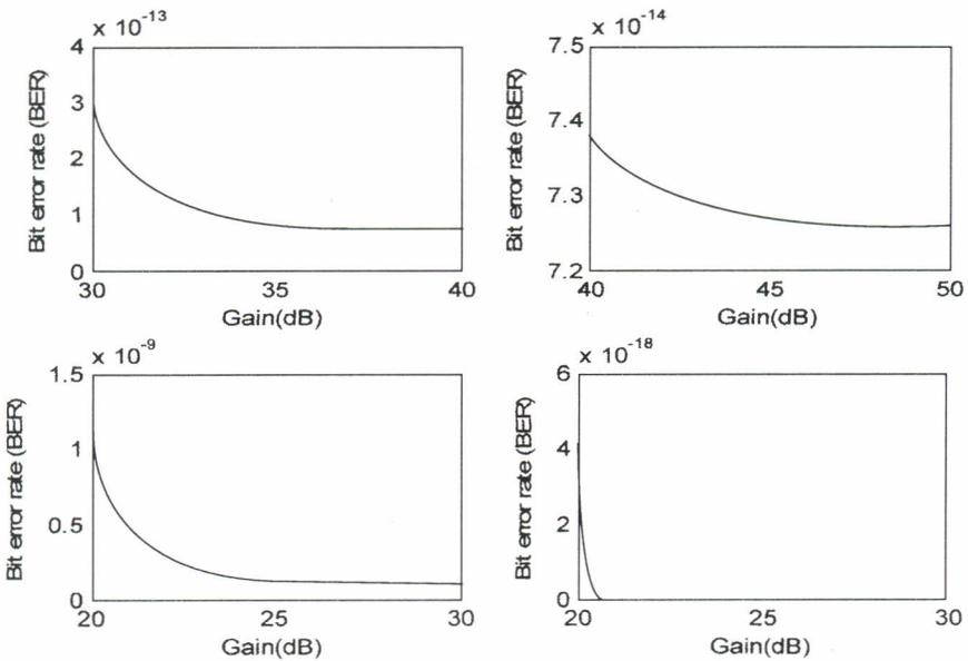
Fig. 3.2 BER vs. Gain curve in 'R' -region, [Fig. 3.2(a)-(d) in cw direction]
