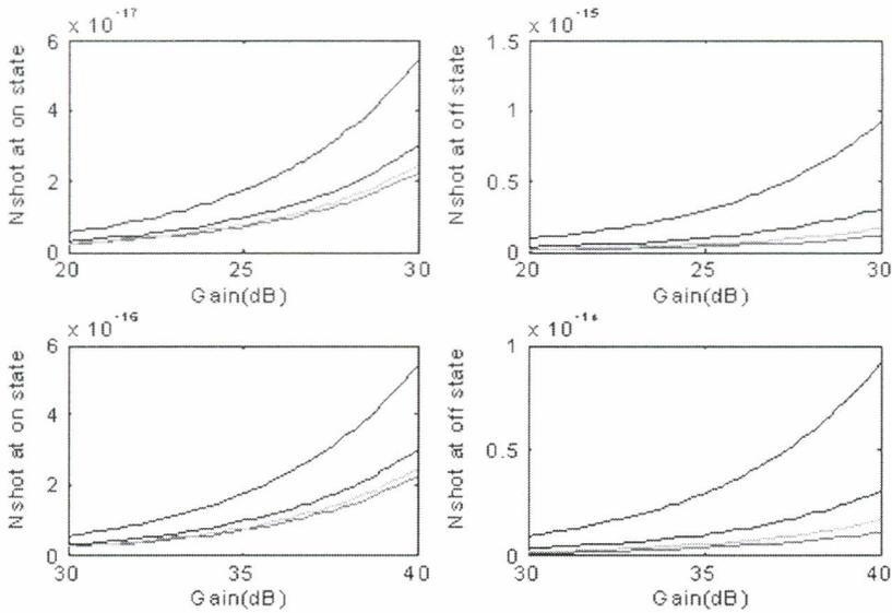
Fig. 3.5 Shot noise vs. Gain curve [ $P_{in}=-50$  (lowest), -48, -45, -40 dBm,  $r=0.04$ ]
