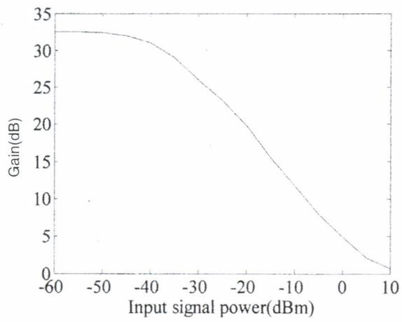
Fig.2.2 Amplifier gain vs. Input power for a typical 1.5 $\mu$ m SLA (figure reproduced) <sup>[6]</sup>
