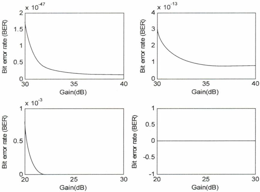
Fig. 3.1 BER vs. Gain curve in 'G', 'R', 'Z' and 'B'-region, [(a)-(d) cw direction]
