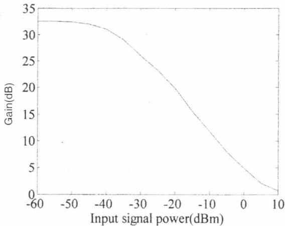
Fig.2.2 Amplifier gain vs. Input power for a typical 1.5 $\mu$ m SLA (figure reproduced) <sup>[6]</sup>
