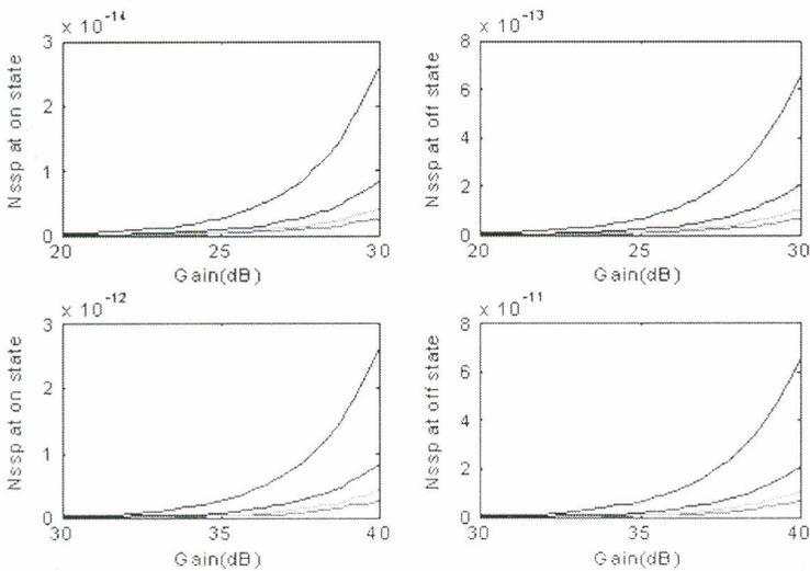
Fig. 3.4 Signal-spontaneous beat noise vs. Gain curve [ $P_{in}=-50$ ~-40 dBm,  $r=0.04$ ]
