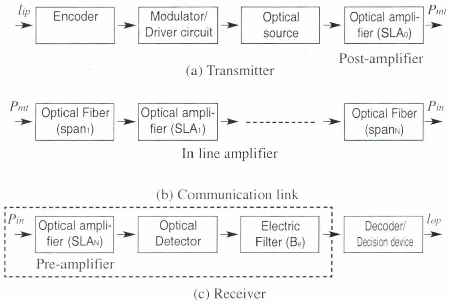
Fig. 2.1 Block diagram of the full ASK-DD system including the amplifier model inside the dotted portion. [9] Here,  $I_{ip}$  =information input at transmitter,  $I_{op}$ =information output at receiver.
