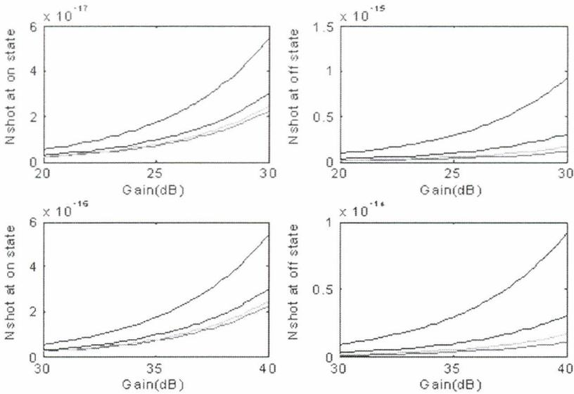
Fig. 3.5 Shot noise vs. Gain curve [ $P_{in}=-50$  (lowest), -48, -45, -40 dBm,  $r=0.04$ ]
