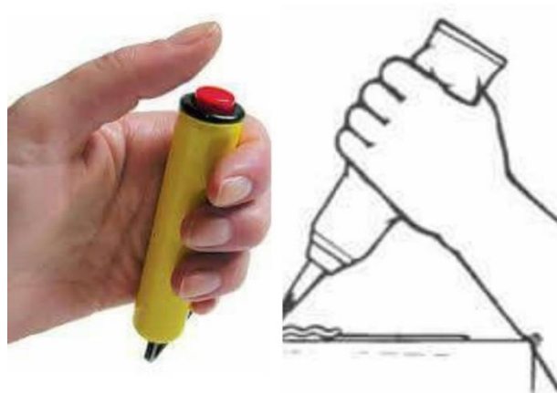
Figure 2.1: Thumb-operated and finger-strip operated pneumatic tool. Thumb operation results in overextension of the thumb. Finger strip control allows all the fingers to share the load and the thumb to grip and guide the tool
