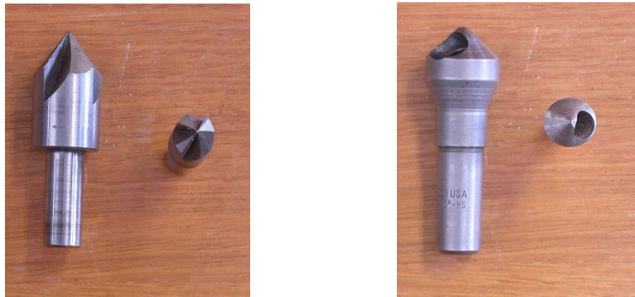
Figure 3.11: Countersinking cutters (4-fluted and non-fluted)
