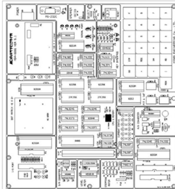
Figure 1.2: MDA-8086 Kit Circuit Diagram
