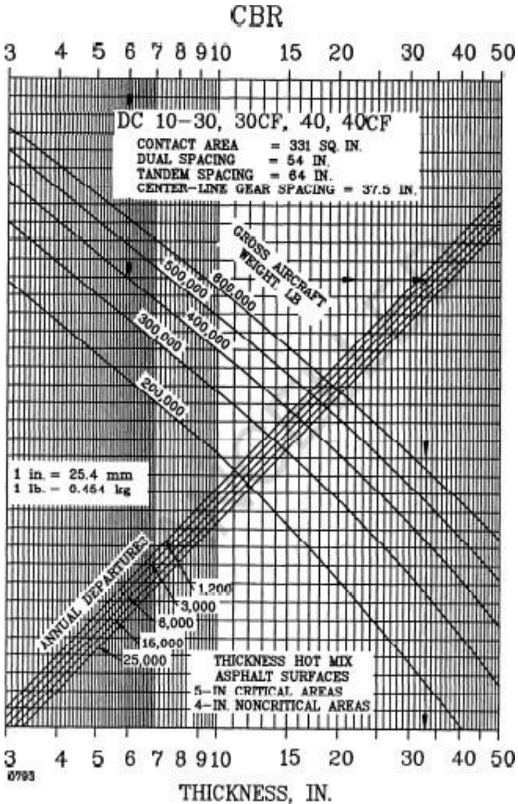
Figure A1.12. Flexible pavement design curves, DC 10-30,30CF, 40,40CF (Source: FAA)
