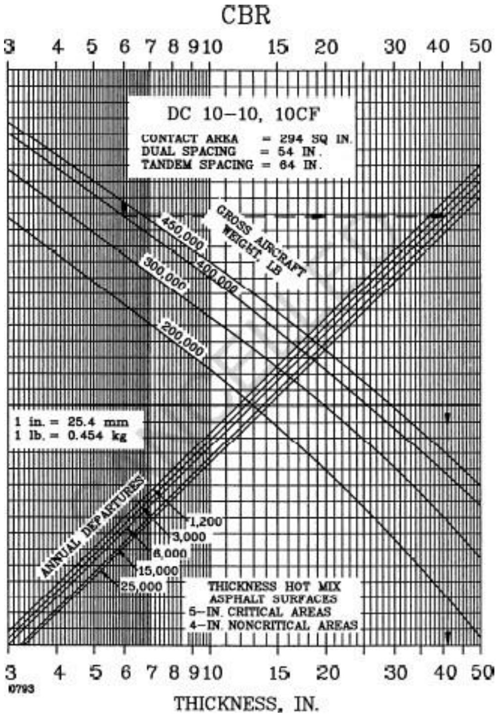
Figure A1.11. Flexible pavement design curves, DC 10-10, 10CF (Source: FAA)
