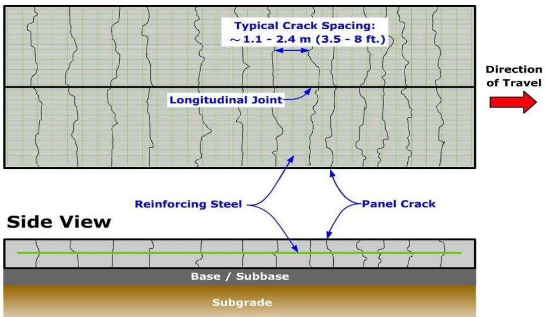
Figure 4.2. Continuously reinforced concrete pavement (CRCP)
