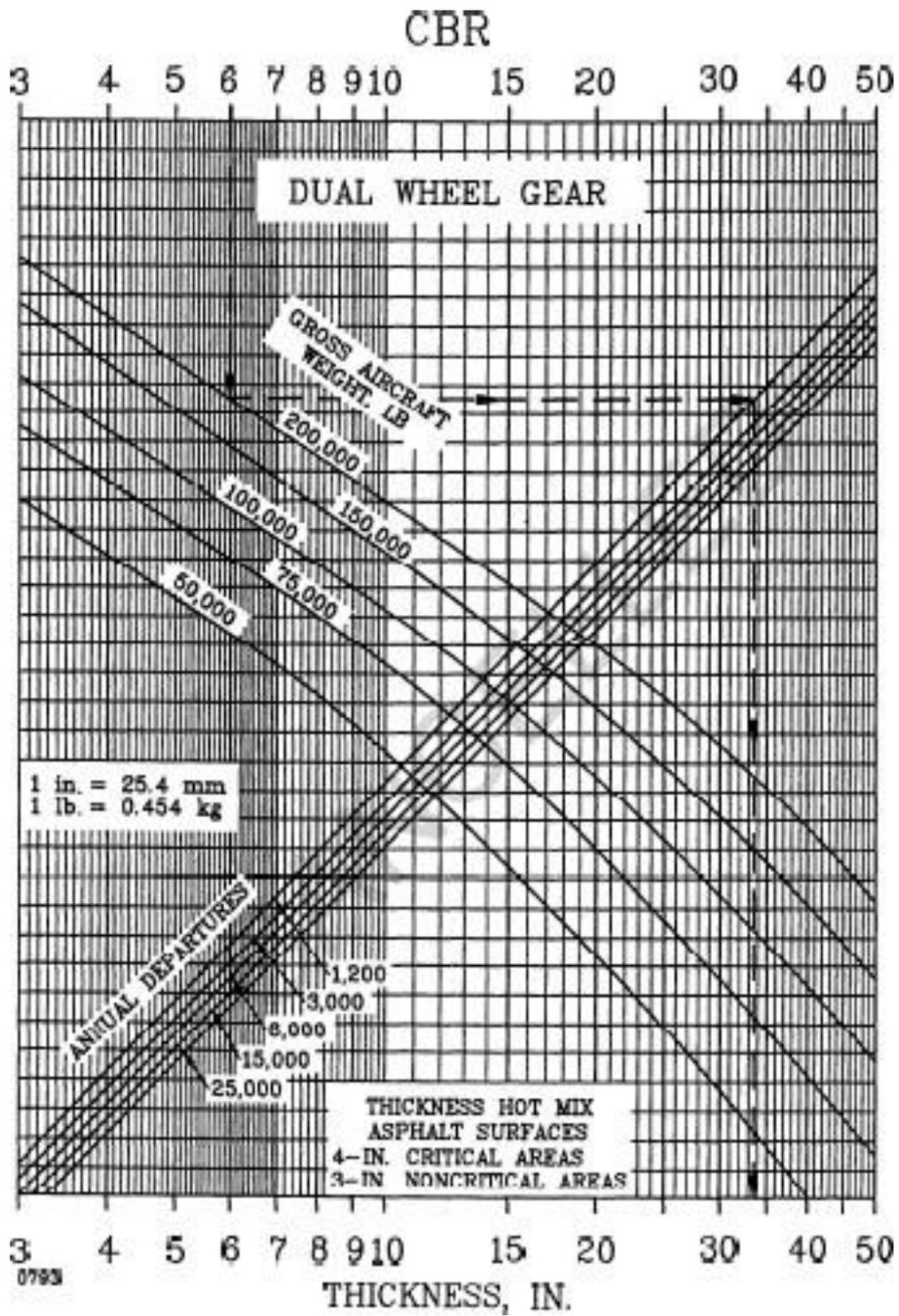
Figure A1.2. Flexible pavement design curves, dual wheel gear (Source: FAA)
