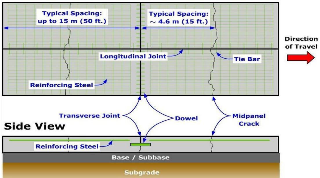
Figure 4.1 Jointed reinforced concrete pavement (JRCP)
