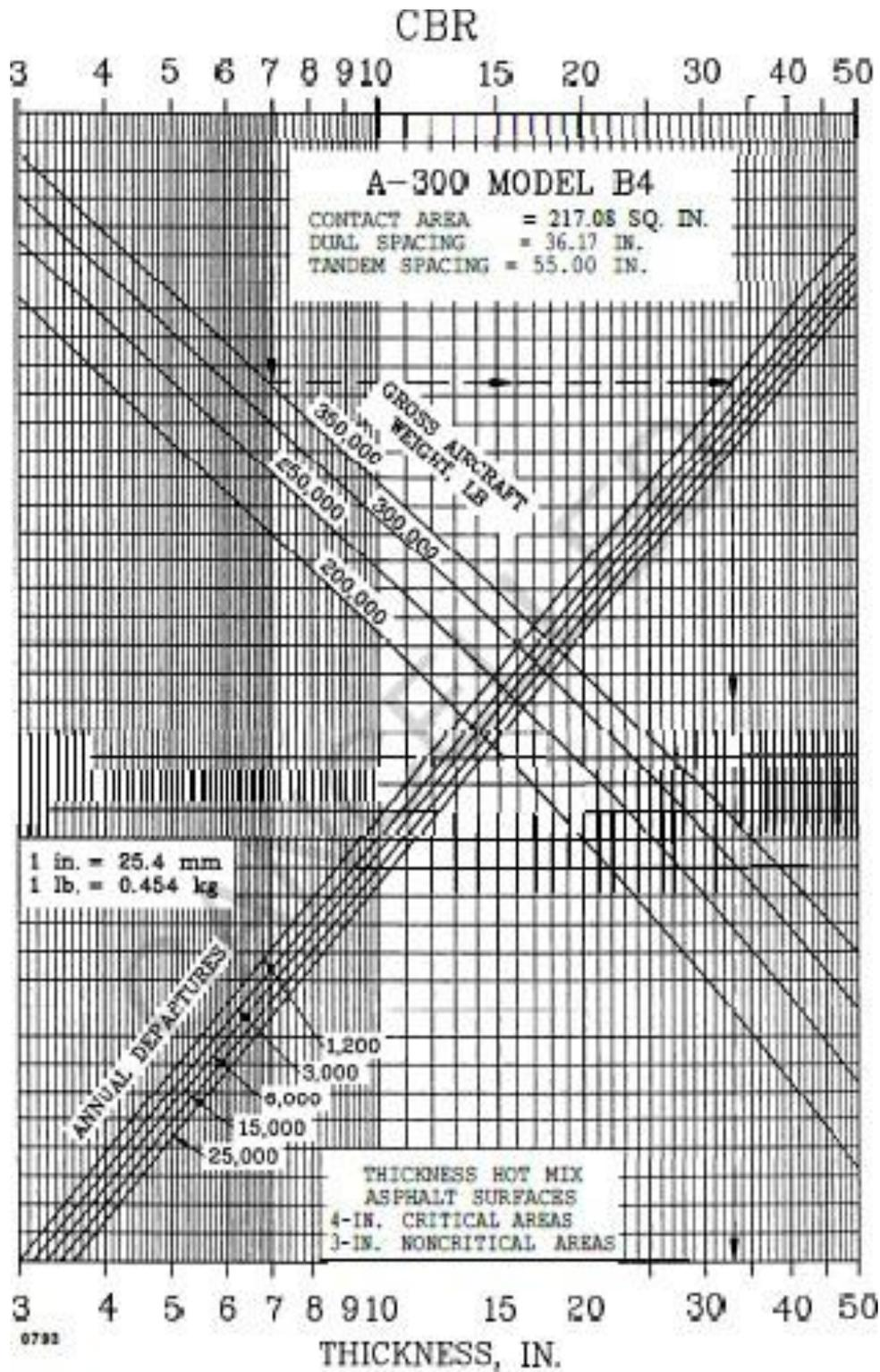
Figure A1.5. Flexible pavement design curves, a-300 model b4 (Source: FAA)
