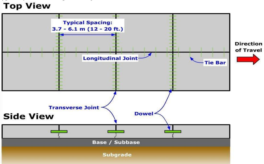
Figure 4.3. Jointed plain concrete pavement (JPCP)
