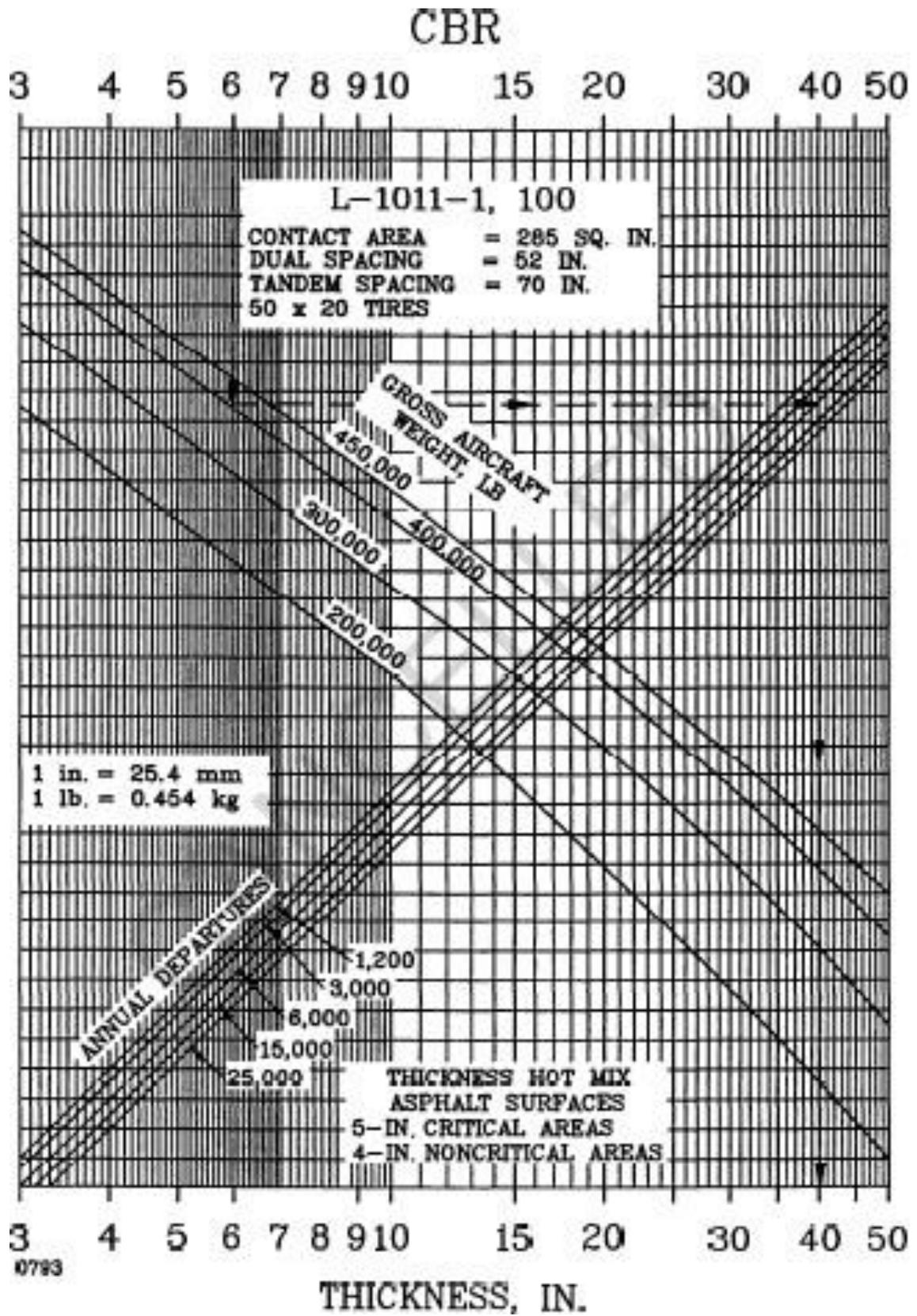
Figure A1.13. Flexible pavement design curves, L-1011-1,100 (Source: FAA)
