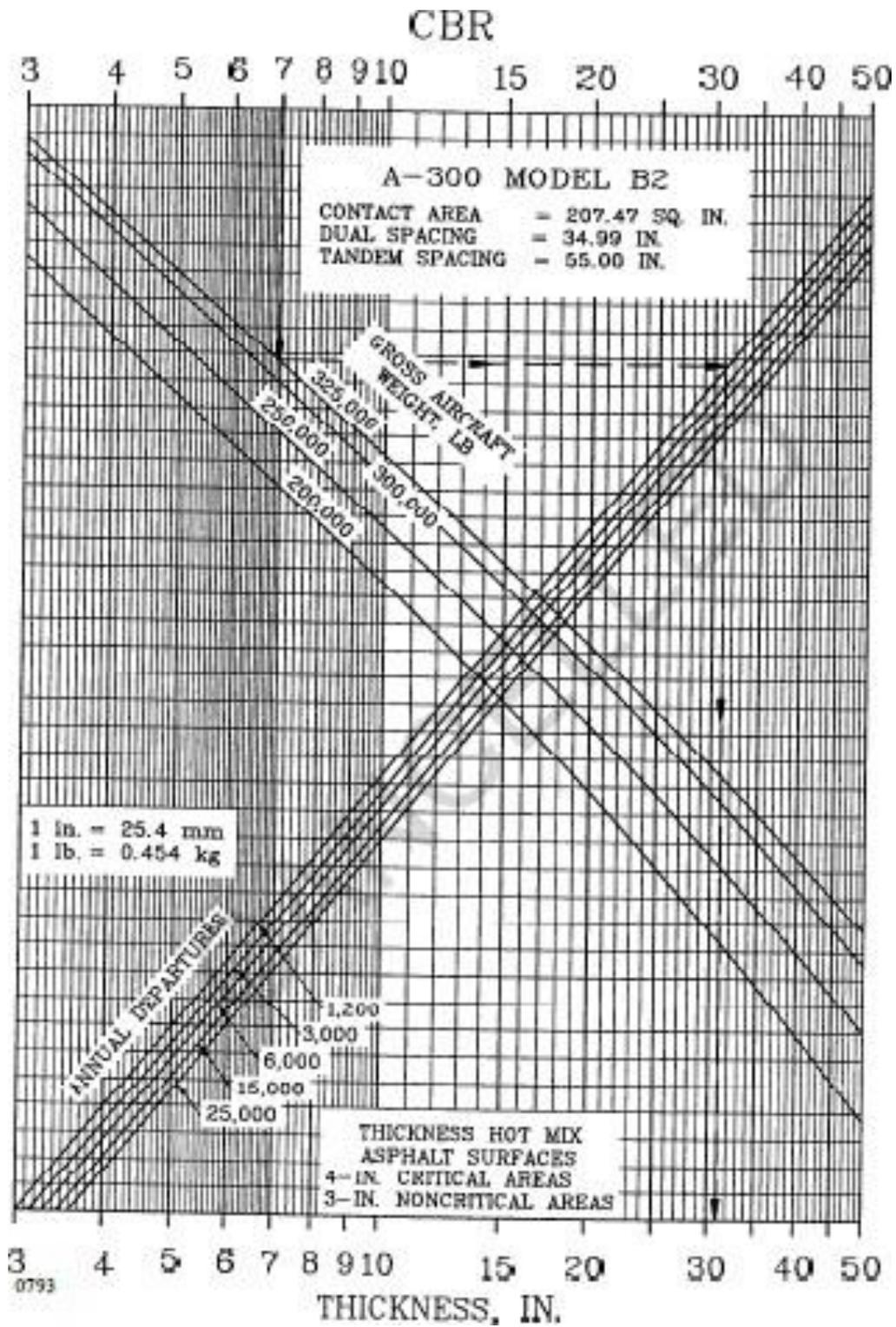
Figure A1.4. Flexible pavement design curves, a-300 model b2 (Source: FAA)
