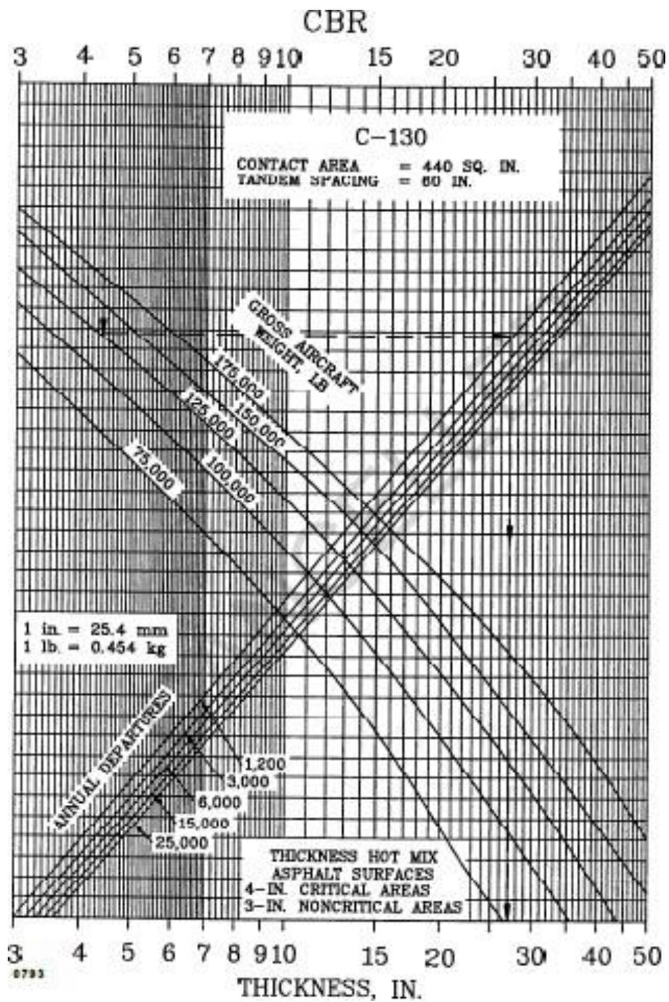
Figure A1.10. Flexible pavement design curves, C-130 (Source: FAA)
