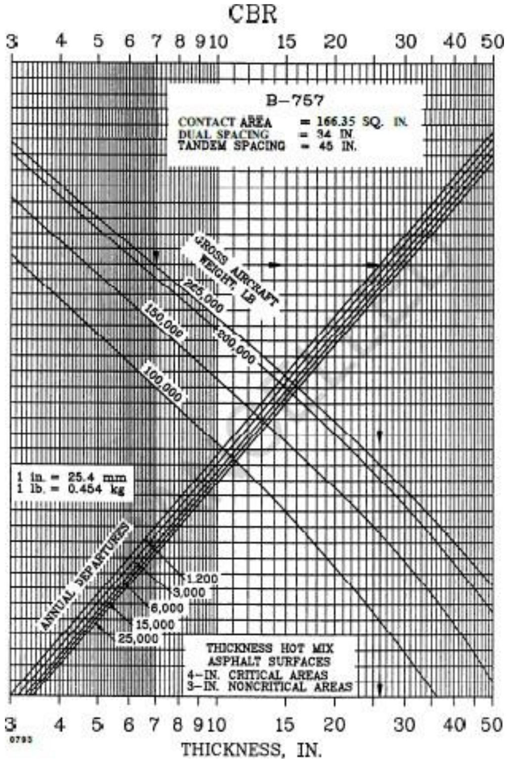
Figure A1.8. Flexible pavement design curves, B-757 (Source: FAA)
