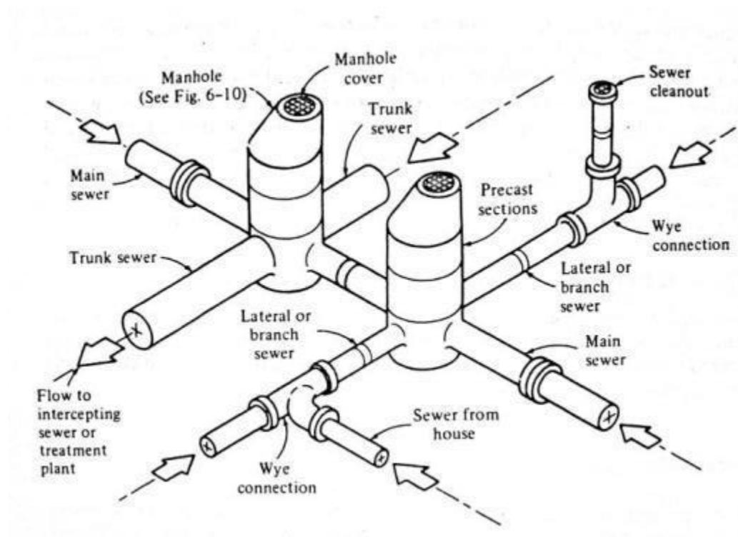
**Figure 6.1:** Definition sketch for types of sewers
