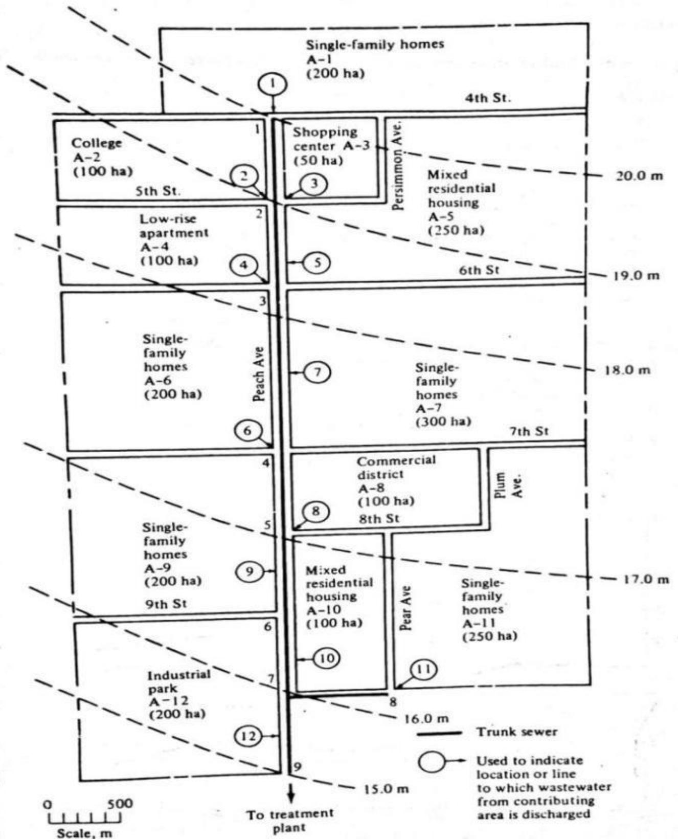
**Figure 6.6:** Contour Map and sewer network of trunk sewer within the contributing area Peak factor for residential areas
