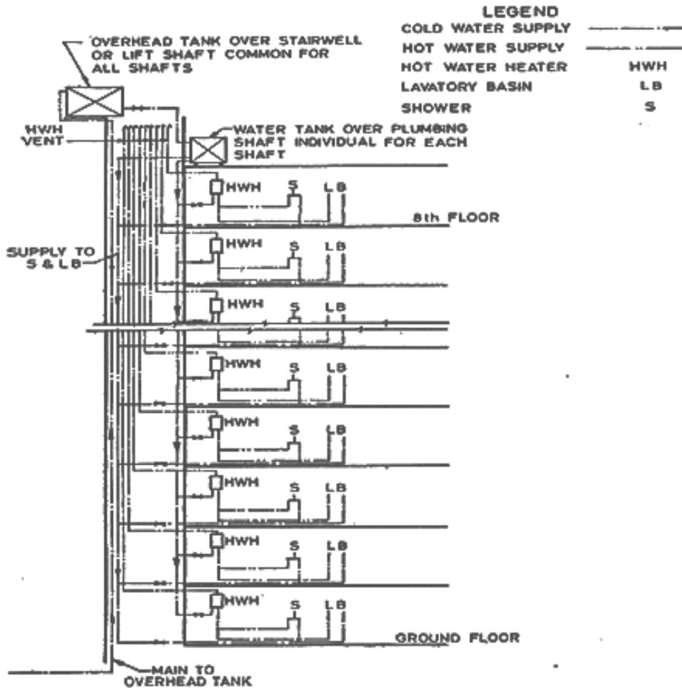
Figure 5.4: Layout plan of the water supply system of a tall building
