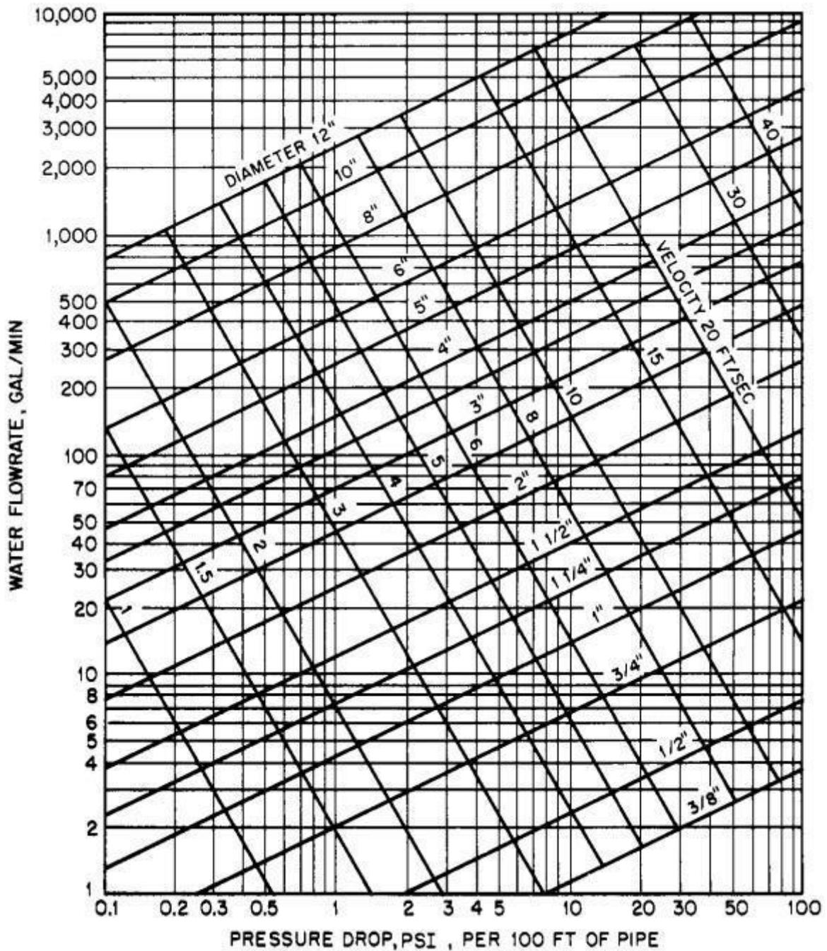
Figure 5.3: Chart for determination of flow in pipes such as galvanized steel and wrought iron that will be fairly rough after 15 to 20 years of use [2]
