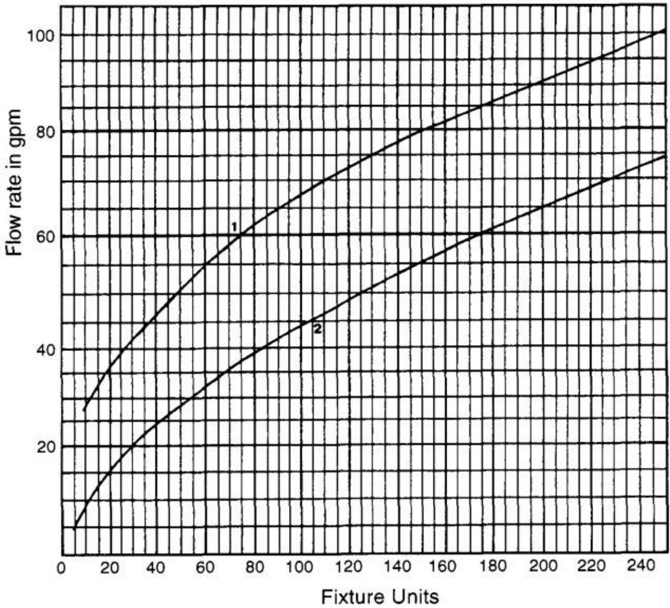
Figure 5.2: Enlarged Scale Demand Load estimation Curve
