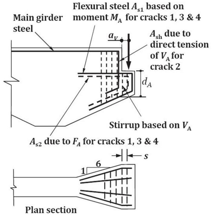
$A_{sh}$  may be provided by extending and bending the main top bar as required. Similarly,  $A_{s1}$  and  $A_{s2}$  may be provided by extending and bending the girder bottom steel.
