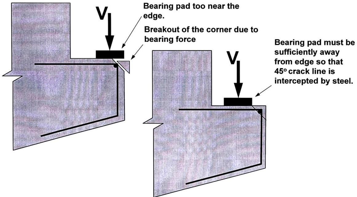
Fig.52 : Clearance requirement around bearing pad near articulation
