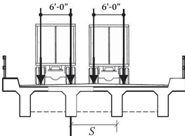
Truck wheel on one side may act directly on an interior girder. The other wheel shall be a distance apart from the girder. Thus full vehicle axle load may not act on one girder. This is considered using a distribution factor. (AASHTO Table 4.6.2.2.2b-1 and 4.6.2.2.3a-1)
