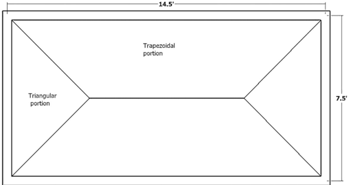
**Figure 11:** Load distribution of slab
