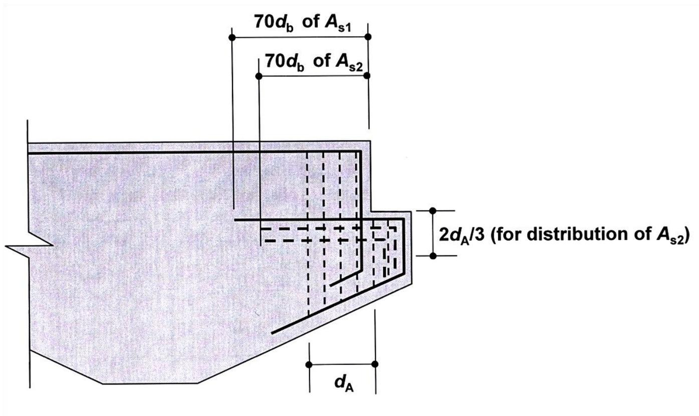
Fig.54 : Reinforcement detailing of articulation
