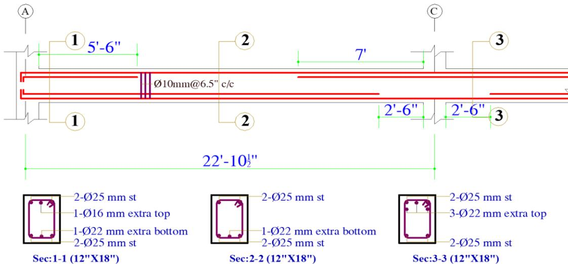
**Figure 17:** Reinforcement detail of beam
