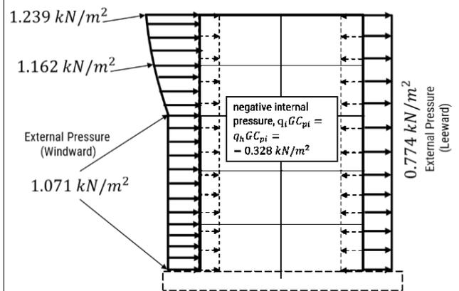
Fig.: Pressure distribution considering negative internal pressure
