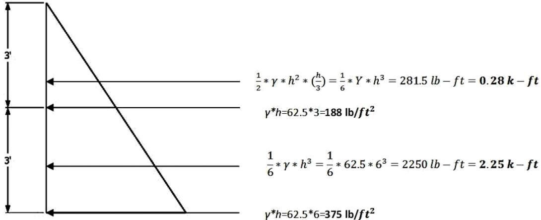
**Figure 8:** Pressure distribution on reservoir wall
