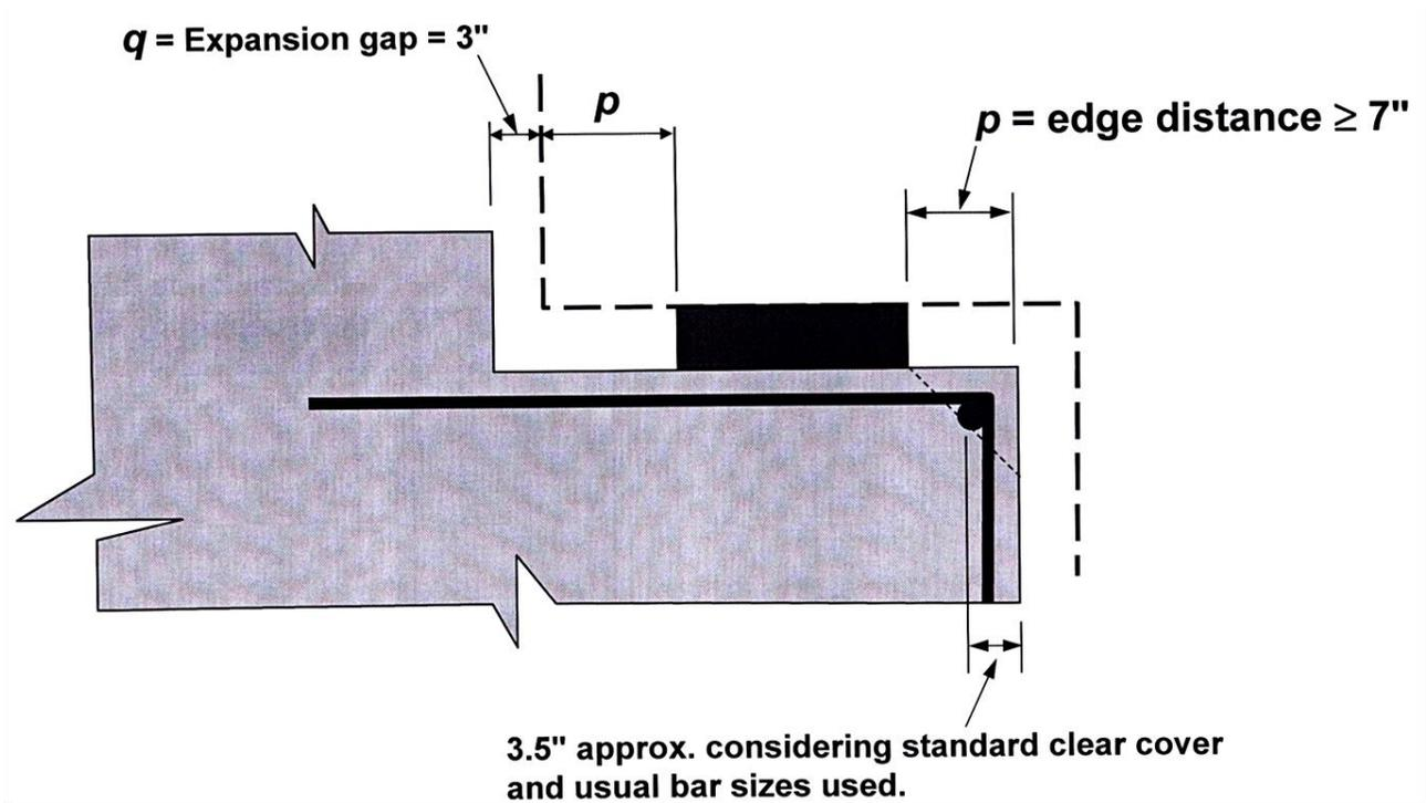
Fig. 53: Expansion gap and edge distance around bearing pad
