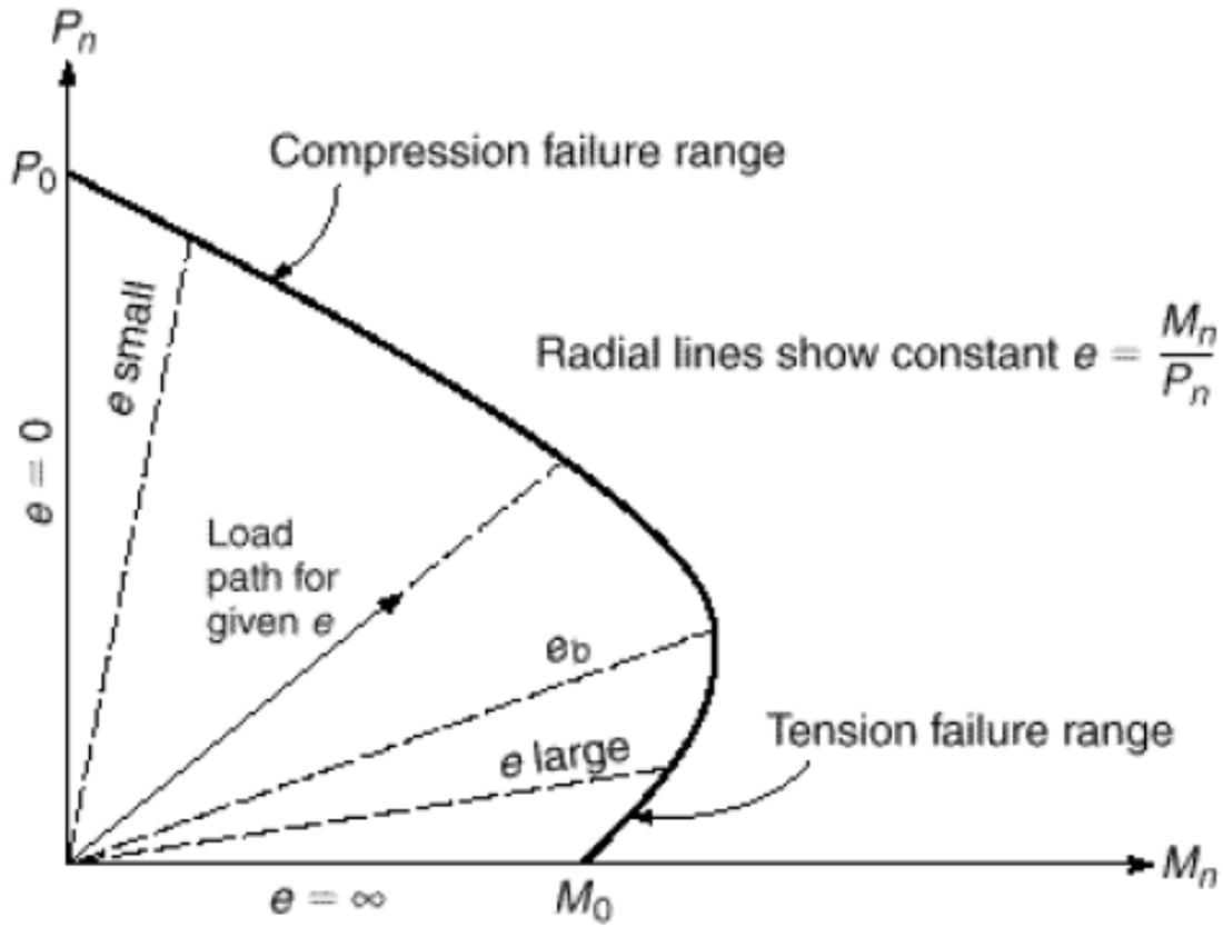
**Figure 19:** Interaction diagram for nominal column strength in combined bending and axial load. (Ref: ACI Code, Design of Concrete Structure, 13<sup>th</sup> edition, Chap-8, P-260)
