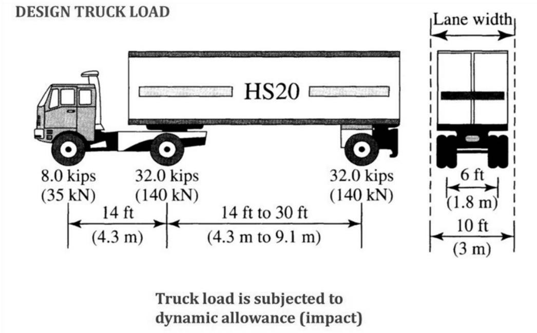
Fig.25: Design Truck load (HS20-516)
