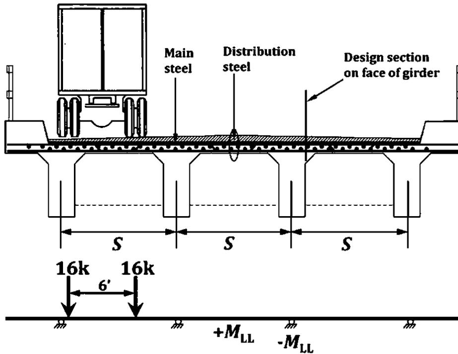
**Detailed analysis can be performed based on influence line to determine the maximum effect.**
