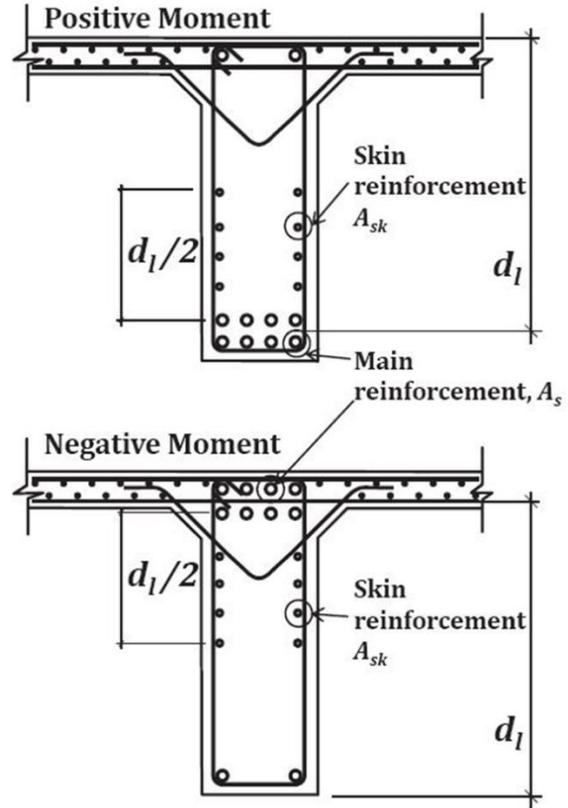
**REINFORCEMENT DETAILING OF T-GIRDERS**
