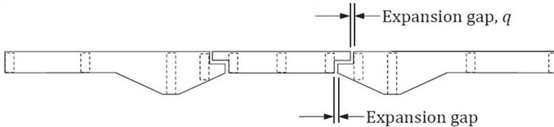
Expansion gap is required to accommodate the thermal expansion-contraction. In Bangladesh seasonal temperature varies between 5 °C to 40 °C. For the purpose of design we take  $\Delta t = 40$  °C.
