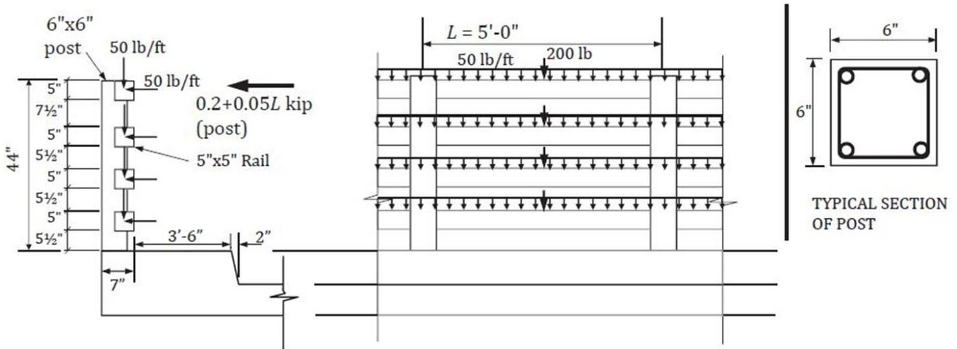
**Each railing shall be designed for 50 lb/ft uniformly distributed load acting simultaneously in both vertical and horizontal direction.**
