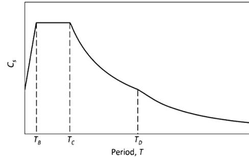
Figure 6.2.25 Typical shape of the elastic response spectrum coefficient C<sub>s</sub>
