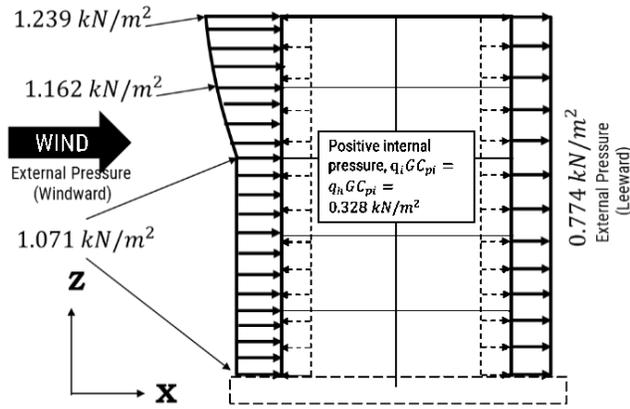
Fig.: Pressure distribution considering positive internal pressure
