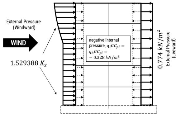
Fig.: Pressure distribution considering negative internal pressure
