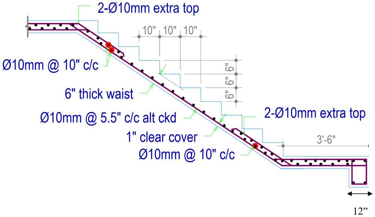
**Figure 6:** Reinforcement details of stair
