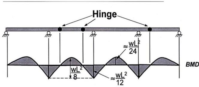
Hinges render the structure determinate:
