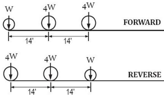
**APPLICATION OF DESIGN WHEEL LOAD: MAX. POSITIVE MOMENT AT SECTION 7**
