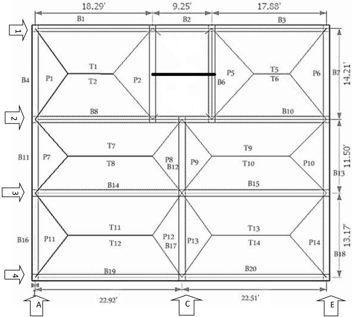
**Figure 16:** Beam layout
