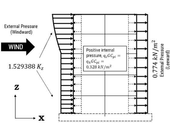
Fig.: Pressure distribution considering positive internal pressure
