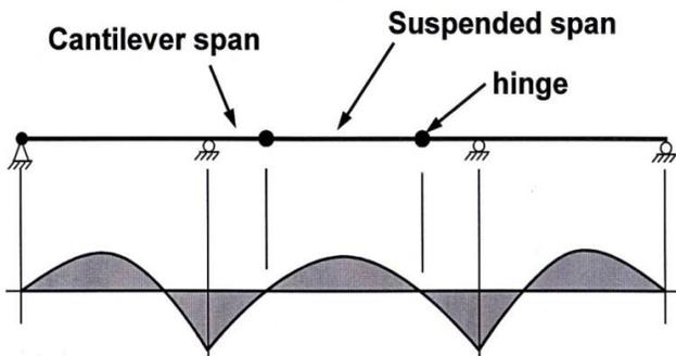
Fig. 15: A bridge having intermediate hinges
