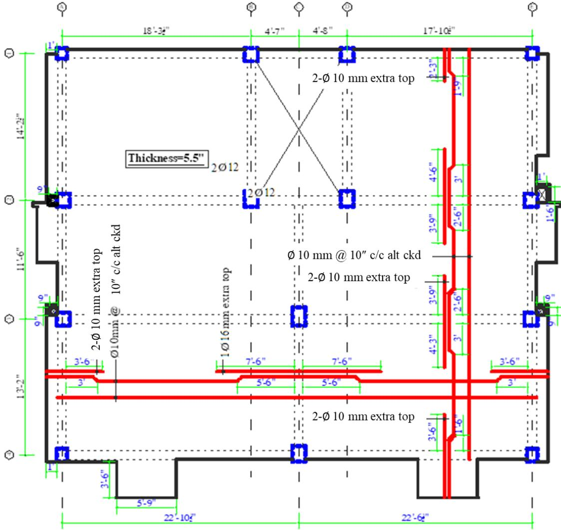
**Figure 15: Typical Reinforcement Details of Slab**
