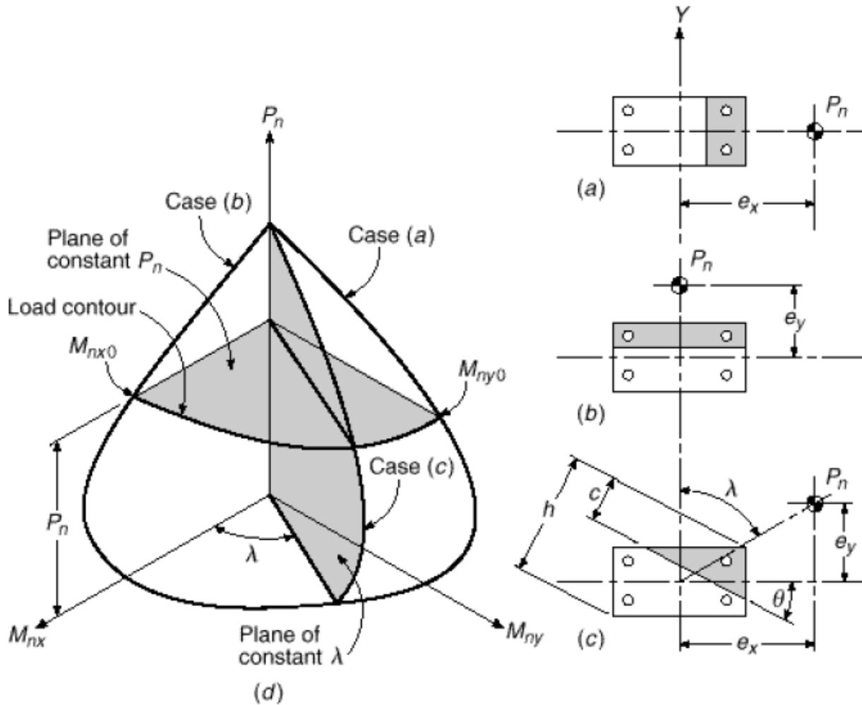
**Figure 18:** Interaction diagram for compression plus biaxial bending a) uniaxial bending about Y axis; b) uniaxial bending about X axis; c) biaxial bending about diagonal axis; d) interaction surface. (Ref: ACI Code, Design of Concrete Structure, 13<sup>th</sup> edition, Chap-8, P-274)
