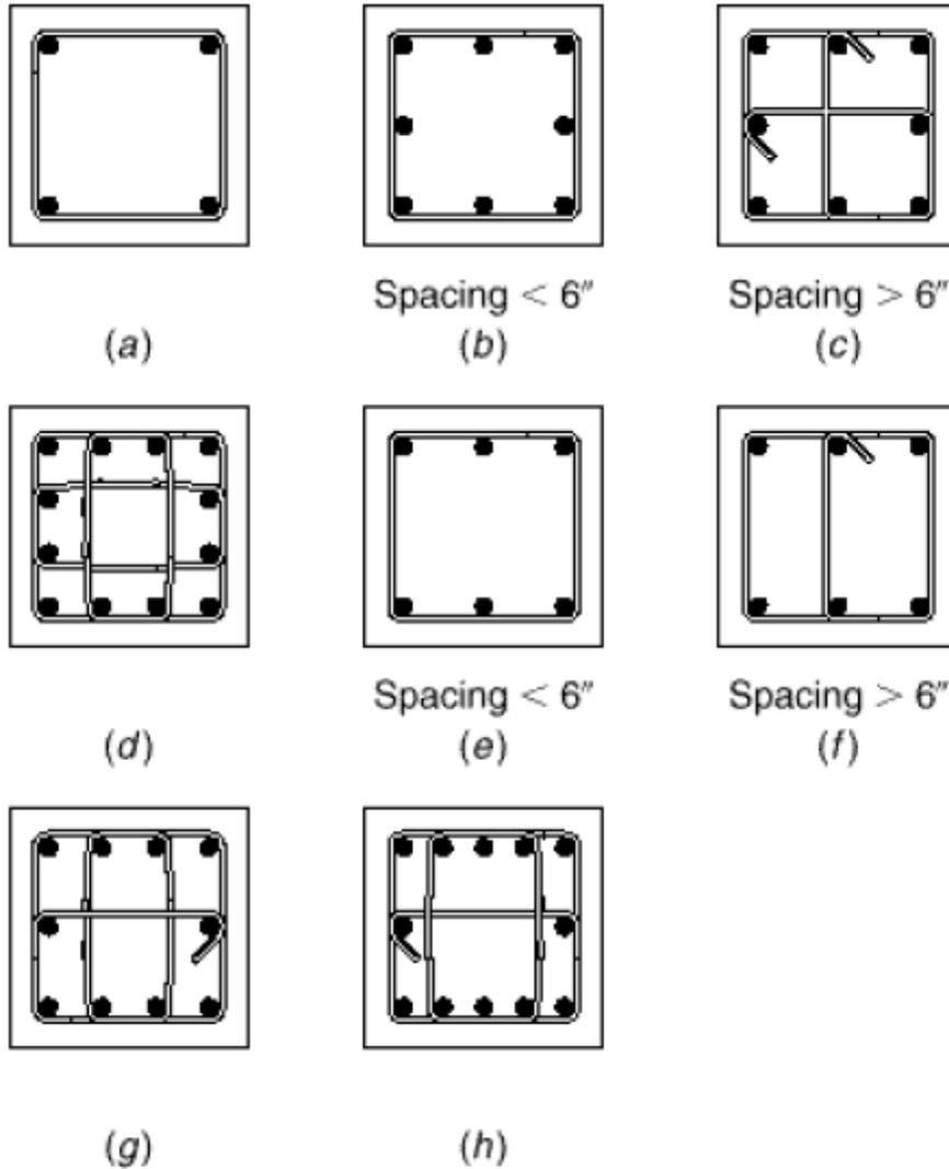
**Figure 22:** Tie arrangement of rectangular column ((Ref: ACI Code, Design of Concrete Structure, 13<sup>th</sup> edition, Chap-8, P-254)
