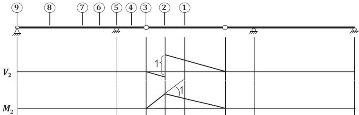
Fig. 39: IL diagram for shear and moment at section 2
