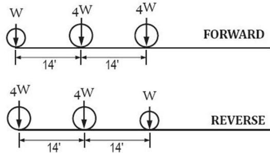
**APPLICATION OF DESIGN WHEEL LOAD: MAX. NEGATIVE MOMENT AT SECTION 7**
