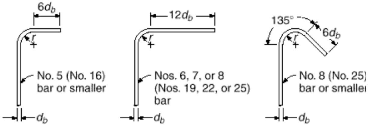
**Figure 23:** Standard bar hook for tie and stirrup. (Ref: ACI Code, Design of Concrete Structure, 13<sup>th</sup> edition, Chap-5, P-177)
