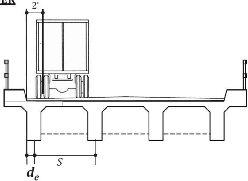
Now prepare the load combination tables for shear and moment. Dead load values shall be recalculated based on revised loading (DC and DW). Live load values may be directly copied from previous load combination tables and combinations may be performed with  $\alpha$  values for exterior girder.
