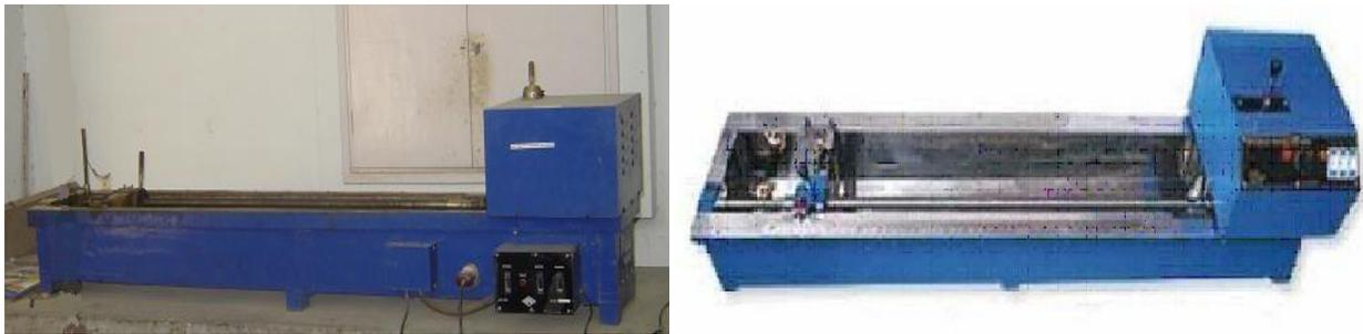
**Figure 2:** Ductility Testing Machine
