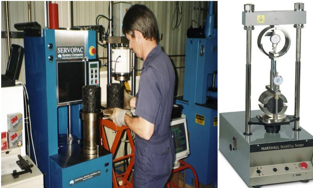
**Figure 17.5** Marshall stability and flow test
