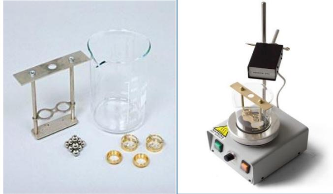
**Figure 12.1** Ring and Ball apparatus
