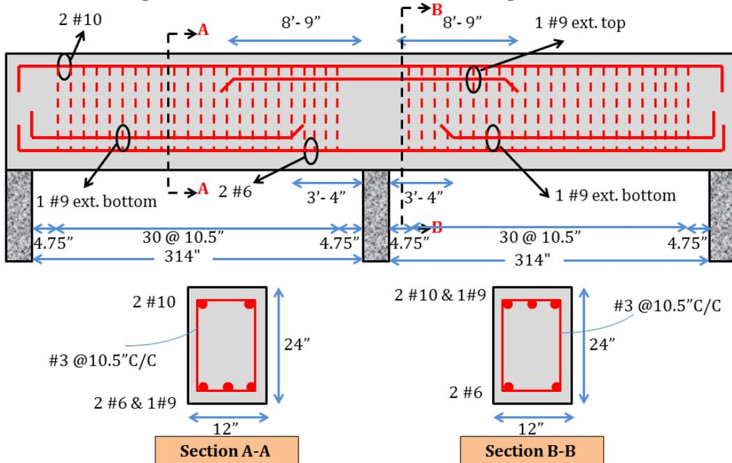
Figure 19: Beam Reinforcement Detailing According to the Design
