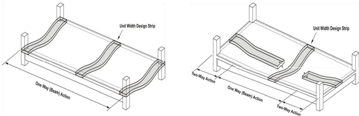
**Figure 2: Slab (a) Supported on two opposite sides only and (b) Supported on all four sides**
