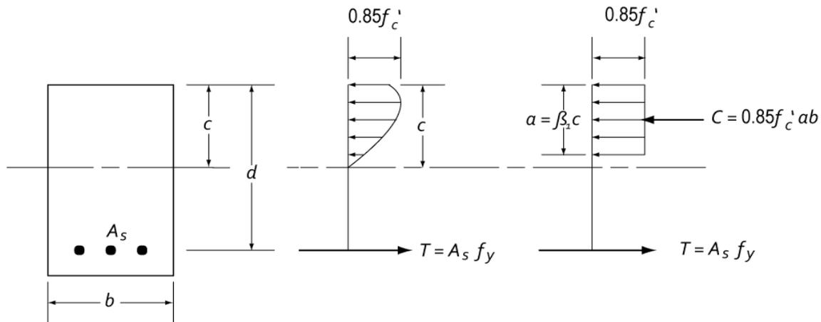
Figure 12: Diagrams for flexure equations
