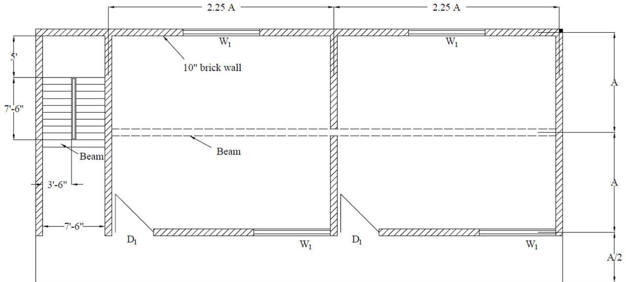
Figure 12: Beam Layout
