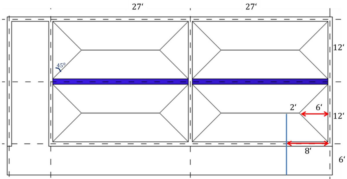
Figure 27: Loads come to Lintel from Slab
