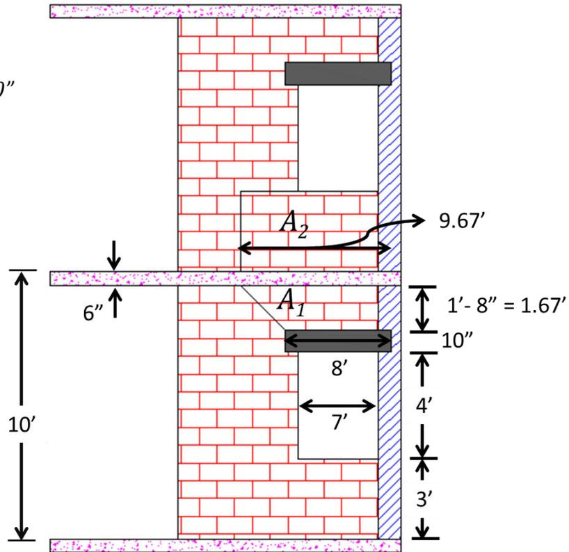
Figure 26: Information necessary to determine lintel load
