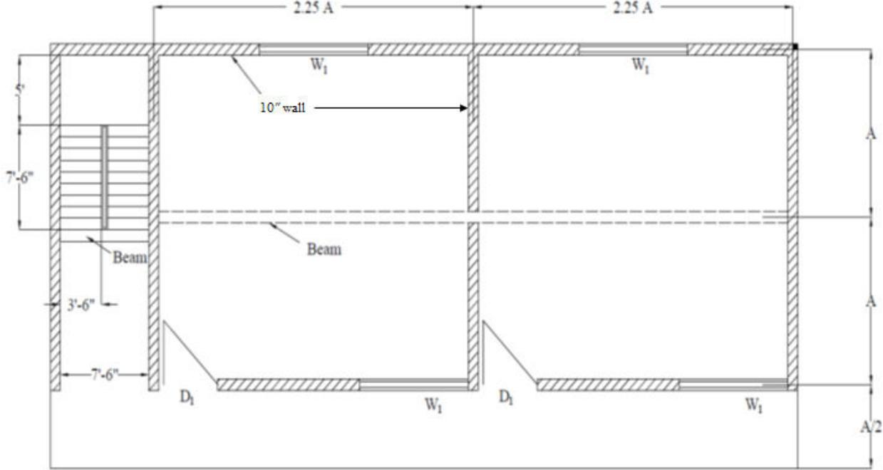
Figure 3: Typical Layout of Load Bearing Building
