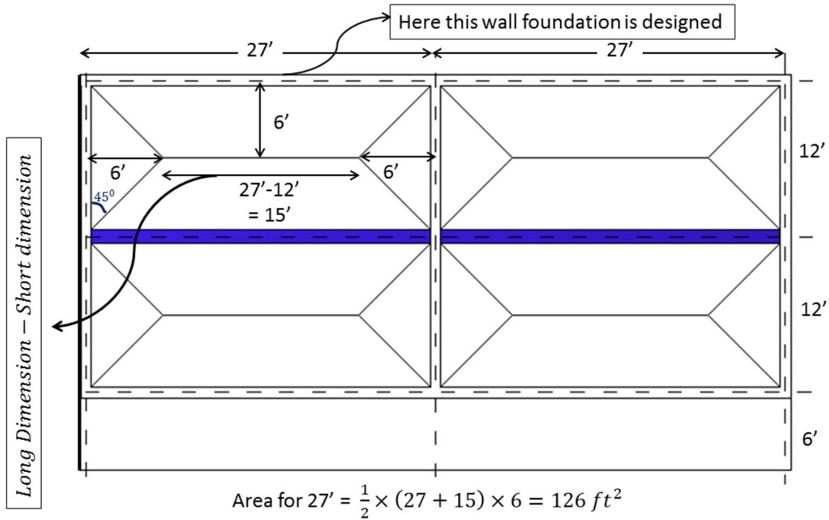
**Figure 30: Contributing area of slab on brick wall**
