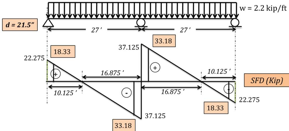
Figure 16: Shear Force Diagram of Beam
