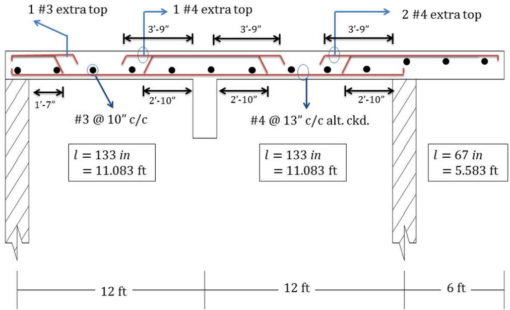
**Figure 9: Detailing at Section 1-1**
