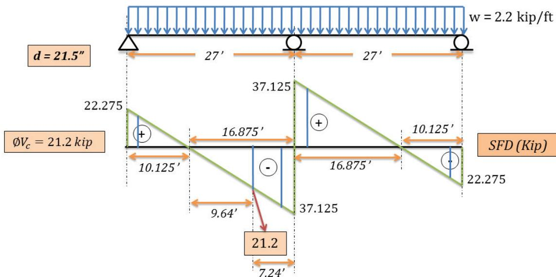
Figure 17: Distance determination where  $V_u = \phi V_c$
