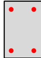
$$\left. \begin{array}{l} M(+ve) = 11.49 \text{ kip-ft} \longrightarrow A_s(+ve) = 0.42 \text{ in}^2 < A_{s,min} \\ M(-ve) = 10.05 \text{ kip-ft} \longrightarrow A_s(-ve) = 0.36 \text{ in}^2 < A_{s,min} \end{array} \right\} = 0.625 \text{ in}^2 (2\#6)$$
