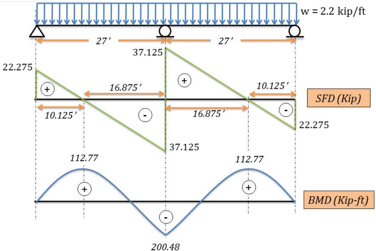
Figure 15: Shear Force Diagram and Bending Moment Diagram
