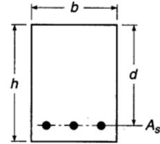
Total Load on Beam,  $w_u = (1.84 + 0.3 \times 1.2) \text{ kip/ft} = 2.2 \text{ kip/ft}$
