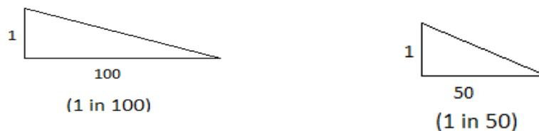
**Fig. 8.3** Typical Slope of Roof Cover
