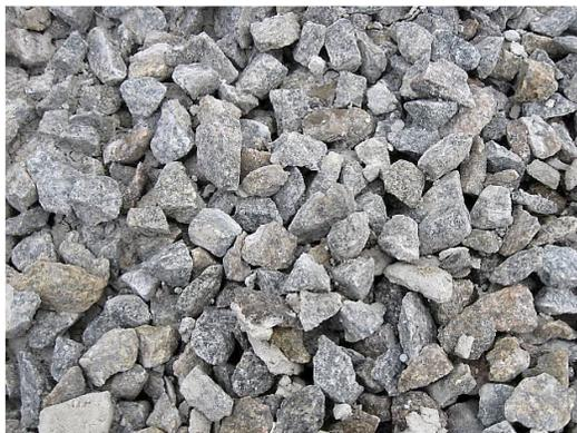
**Fig. 9.4** Coarse Aggregate
