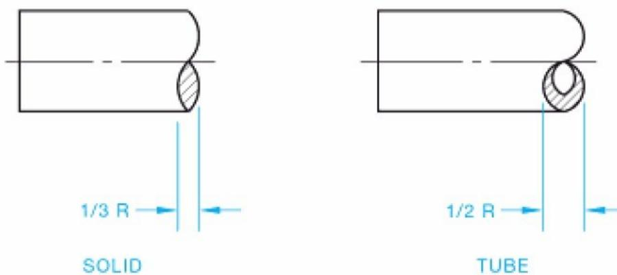
Cylindrical conventional breaks for a solid and tube;
