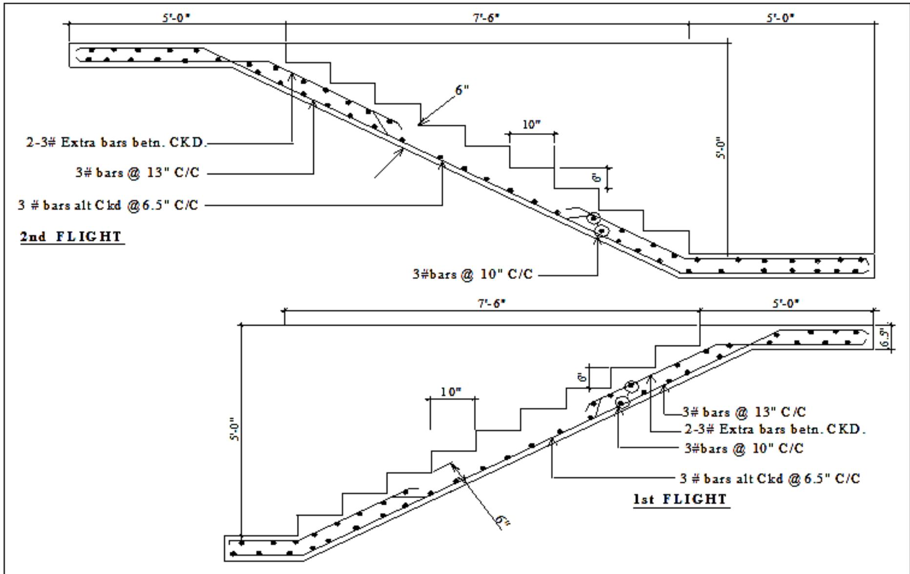
**REINFORCEMENT DETAILING OF STAIR**
